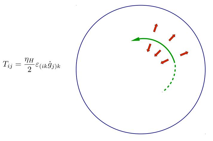
• Constant stirring creates an orthogonal static force, non dissipative
